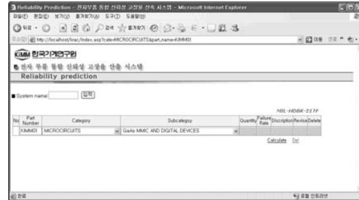
Fig. 3. Selection of the reliability prediction item (on MIL-HDBK-217F N2).
