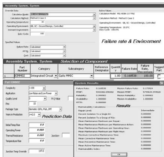
Fig. 6. The result of the failure rate calculation of the electronic component by using Relex.
