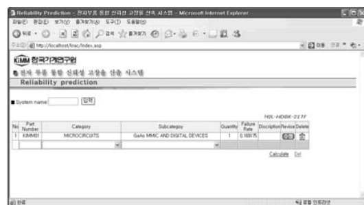
Fig. 5. Output of the result of the failure rate prediction.
